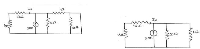
$10\Omega$  is redundant hence the circuit will get modified. As shown above.
