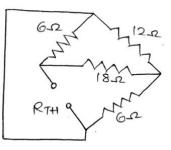
$6\Omega$  resistor is parallel with  $12\Omega$  gives resultant resistance  $4\Omega$
