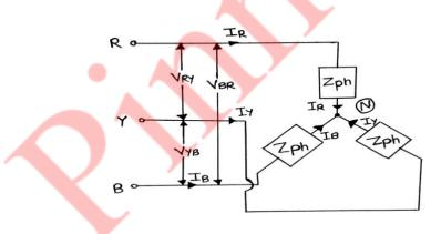
Since the system is balanced, the three-phase voltages  $V_{RN}$ ,  $V_{YN}$ ,  $V_{BN}$  are equal in magnitude and differ in phase from one another by 120°.
