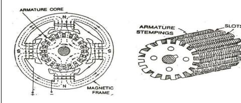
The armature core of a DC generator or machine serves the following purposes.
